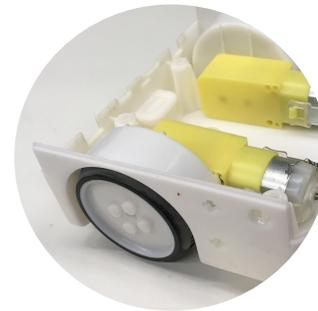
Thymio moves thanks to its two wheels, each driven by a motor.
