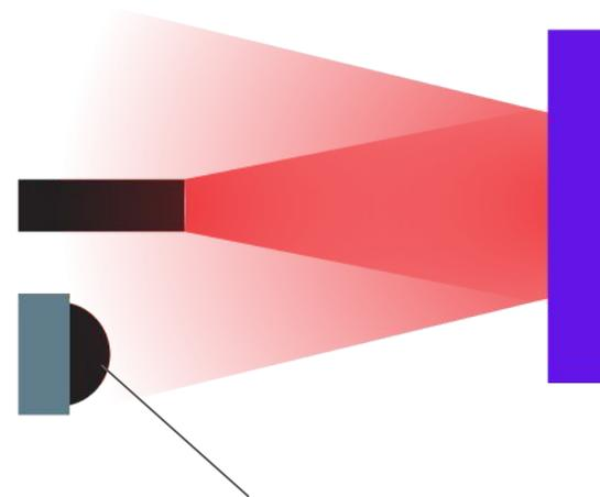
Presence of an object, detection of the return signal
