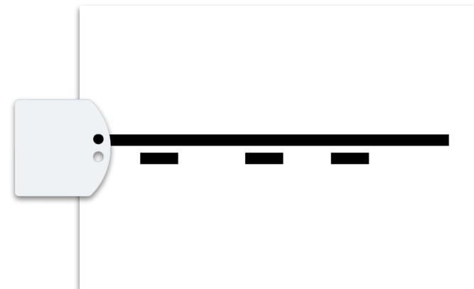
Thymio can therefore be programmed to follow a narrow line using only one of its sensors, and use the other sensor separately to program another action.
