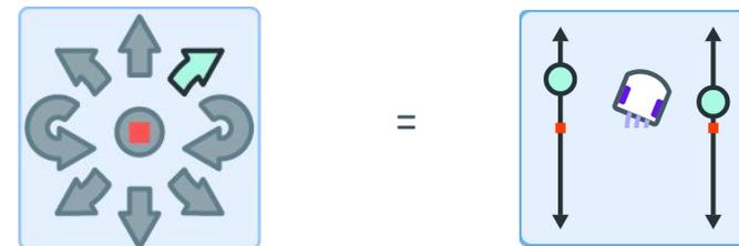
The setting of the wheel speed allows the execution of different curves.
